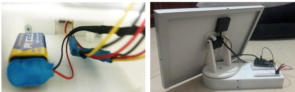
Figure (8) Installing the Arduino and connecting the motor and battery wires
