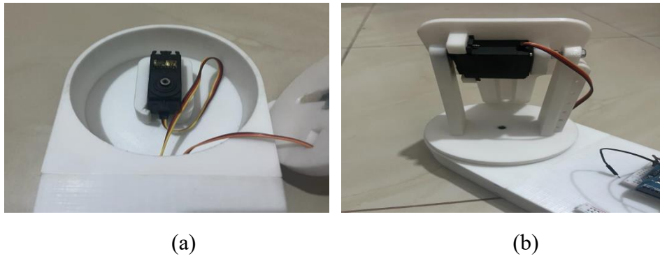
Figure (7) Bottom motor installation responsible for: a) Azimuth angles, b) Altitude angles
